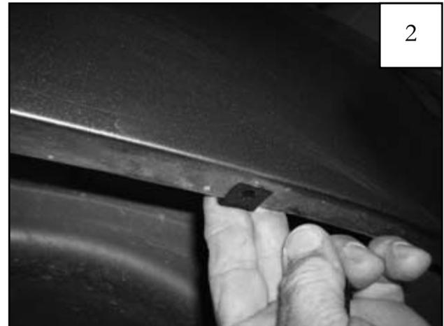
Center a supplied Clip (CL1-0022) over the two holes in Step 1. Clips may need to be adjusted to align with holes in flare. *Note: The raised collar on the Clip should face upward into the interior of the fender.*
