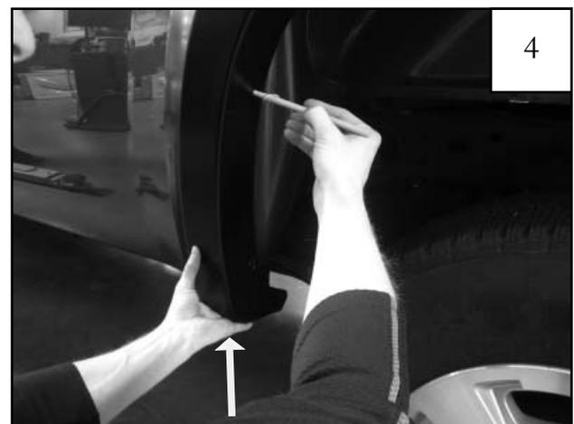
Pushing upward on the flare to ensure proper positioning, use a grease pencil to mark four hole locations. Remove screws installed in Step 3 and remove flare.
