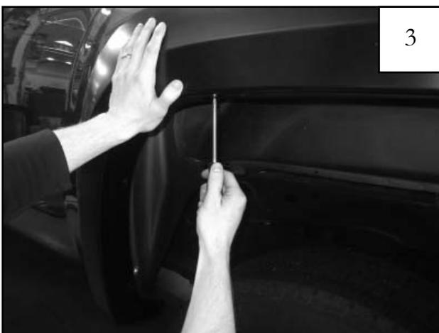
Align flare on vehicle and start a supplied screw (SW1-0058) through the two uppermost holes in the flare and into each clip installed in Step 2. **DO NOT FULLY TIGHTEN SCREWS AS THEY WILL BE UNINSTALLED**
